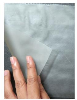
Figure 1. A visual image of starch based self-supporting CS\_PVA\_GA film with added antimicrobial agent SP at 1.791 g/100 g polymer.
